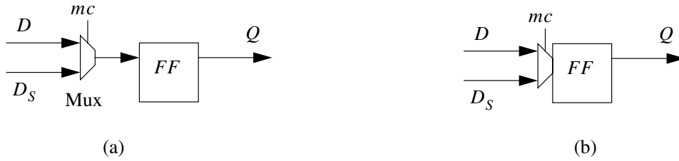
Figure 11.2 A multiplexed-input scan flip-flop (Williams and Angell, 1973) (© 1973 IEEE). (a) An example implementation, and (b) its symbol
