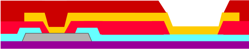
Deposit, pattern, and cross-link second layer of BCB passivation (BCB2).
