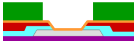
Deposit, expose and develop plating resist.
