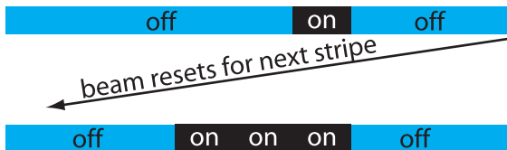
Figure 11–6. Turning the electron beam on and off as it travels from left to right creates the entire pattern, one row at a time.
