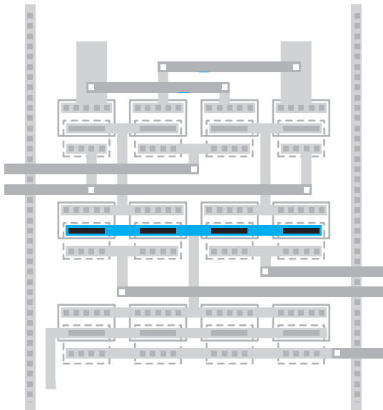
Figure CS2-11. Common emitter connection through our diff pair.
