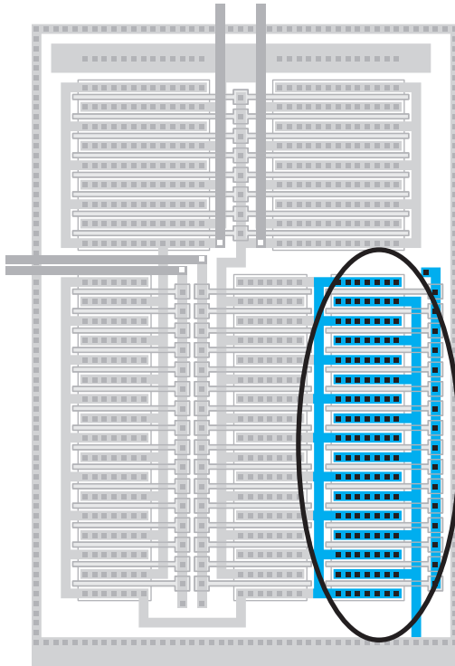
Figure CS1–26. Rotating M5 by 90 degrees would allow better current flow from the far end of the device.
