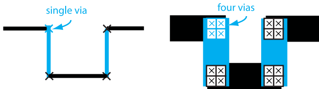
Figure 8–3. Thicker wire allows additional vias between metals.
