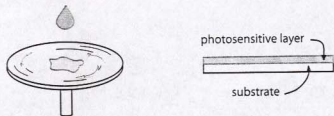
Figure 2-11. Substrate is coated evenly with photosensitive resist by dropping the chemical onto the spinning wafer.
