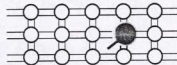
Figure 1-12. One silicon atom has been replaced by an atom containing one extra electron. We see an extra electron that has no bonding partner.
