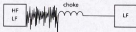
Figure 8-12. Low frequency seems to have an intergalactic Multi-Pass. It is allowed through any inductor at any airport. The high frequency is choked at the inductor.
