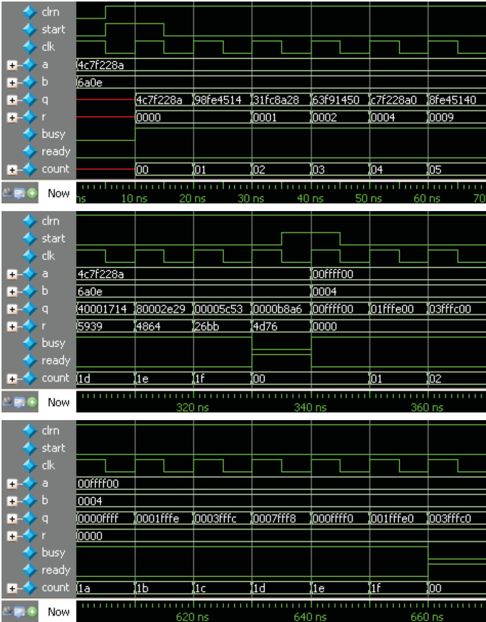
Figure 3.21 Waveform of a restoring divider
