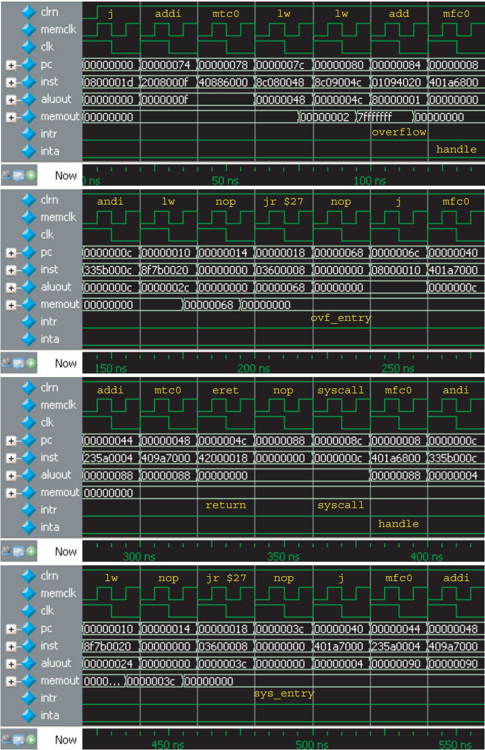
Figure 6.12 Waveform of overflow and system call exceptions
