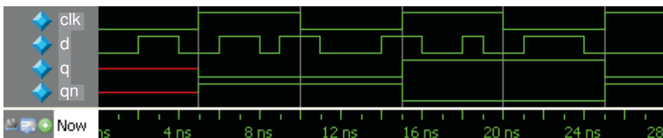
Figure 2.20 Waveform of an academic D flip-flop
