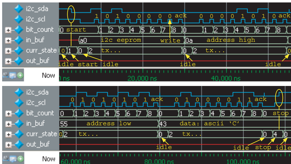
Figure 14.48 Waveform of I2C EEPROM write
