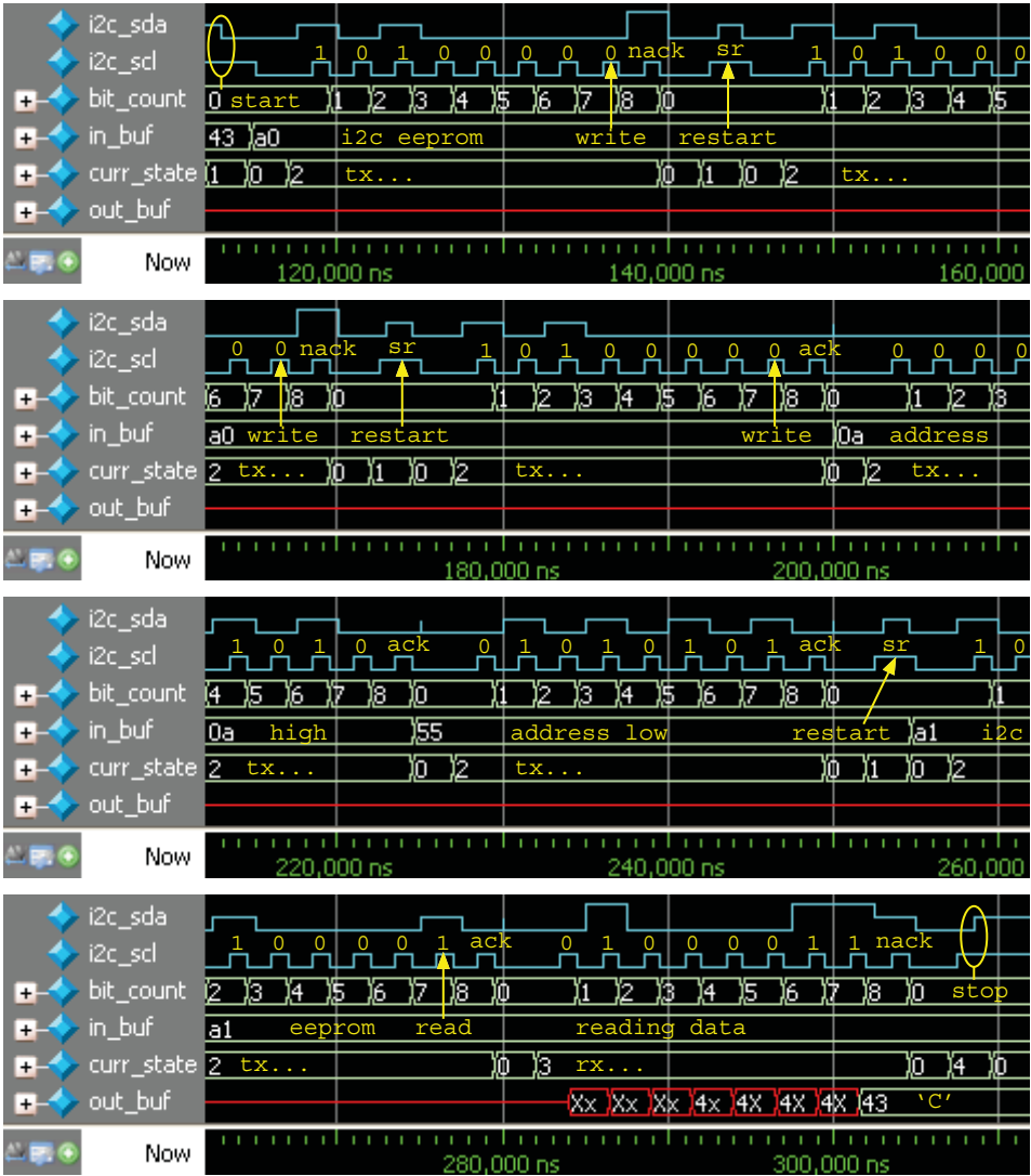
Figure 14.49 Waveform of I2C EEPROM read
