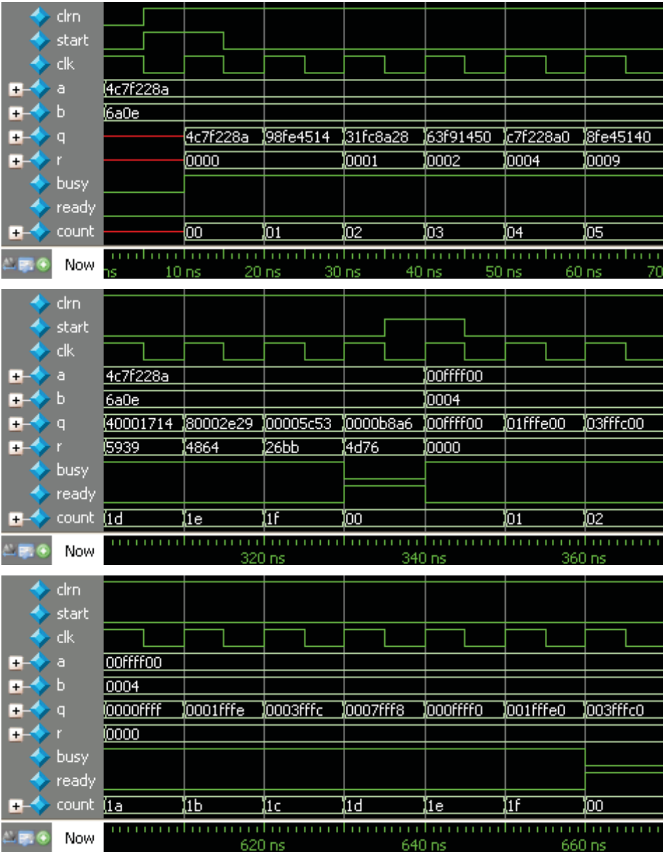
Figure 3.23 Waveform of a nonrestoring divider
