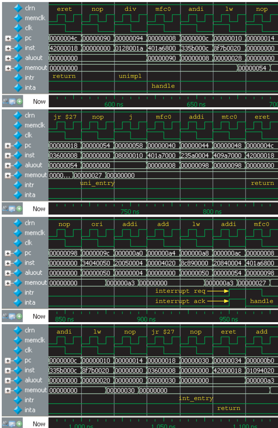
Figure 6.13 Waveform of unimplemented instruction exception and interrupt
