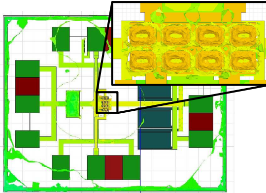
Figure 4.16: Simulated electric fields at 100 MHz. The darker yellow regions correspond to the regions where the value of the electric field is high i.e. where the P+ guard rings of the transistors are located.
