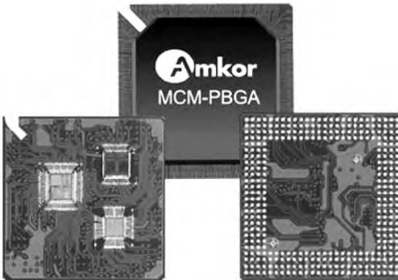
Figure 5-5(c). Laminate MCM-L in Molded BGA Package. Top—Molded Package; Left—Wire Bonded ICs; Right—Bottom of Package
