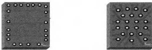
Figure 1-8(a). Peripheral and Area Array I/O formats
