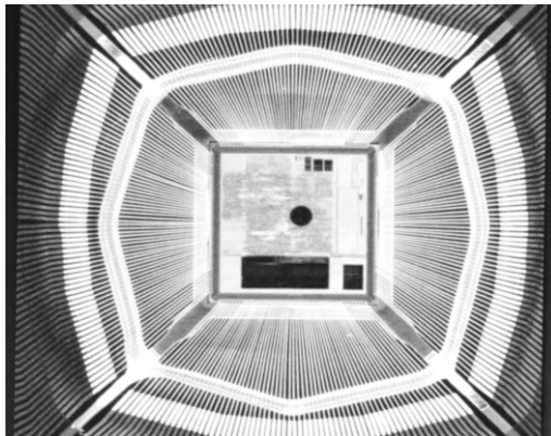
Figure 8-17. PBGA Showing Fan Out of Package Pads and Long Loop Wire Bonds
