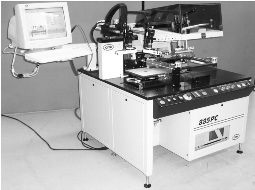
Figure 13-6. Automatic Thick Film Screen Printer
