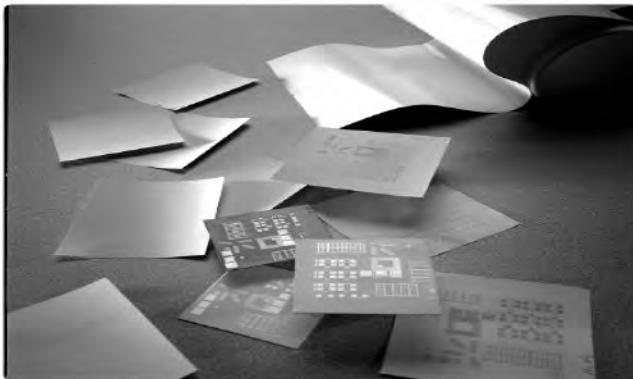
Figure 14-4. Unfired (“Green”) Ceramic Tape
