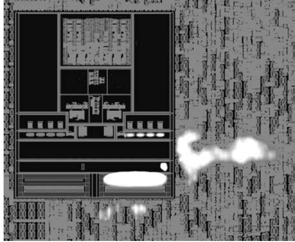
Figure 4.49 Emission microscope (EMMI) tool example of latchup propagation. Source: [82]. Reproduced by permission of IBM.
