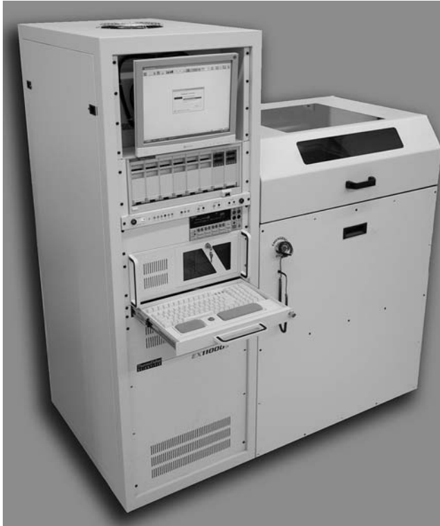
Figure 4.25 Commercial latchup test system (Oryx Instruments 11000 EX, presently Thermo Fisher Scientific).
