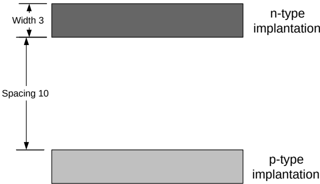
FIGURE 17.7 Design rules for implantations of opposite conductivity type.
