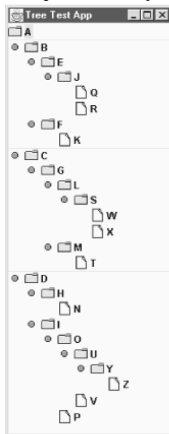
Figure 17.6. The JTree representation of the tree in Figure 17.3
