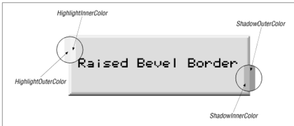
Figure 13.5. The four colors of a bevel border
