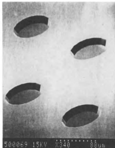
90 \mu\text{m} OPENINGS in POLYIMIDE
