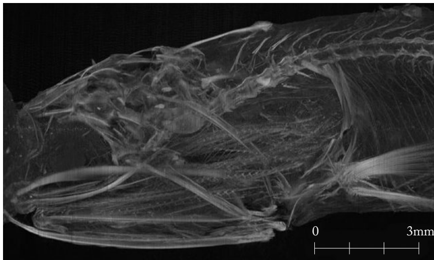
Figure 6.3: An example of X-ray CT image (small fish) taken by the integration-type SOI sensor (INTPIX4) with 9.5 keV synchrotron X-ray. The detector has 500 \mu\text{m} thick FZ sensor and it is operated at detector voltage of 220 V.
