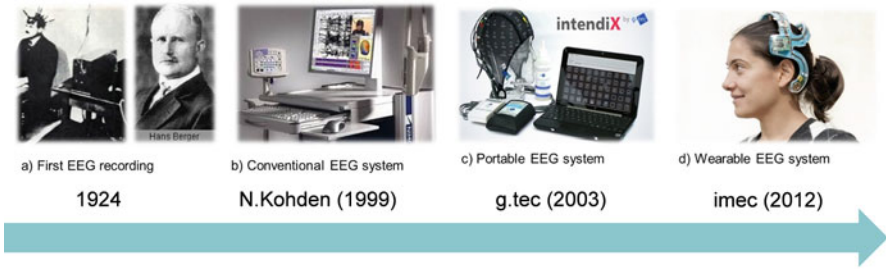
Fig. 7.3 Evolution of EEG acquisition systems toward small size and low power. This trend reflects people’s growing needs for care, cure, and prevention of chronic diseases
