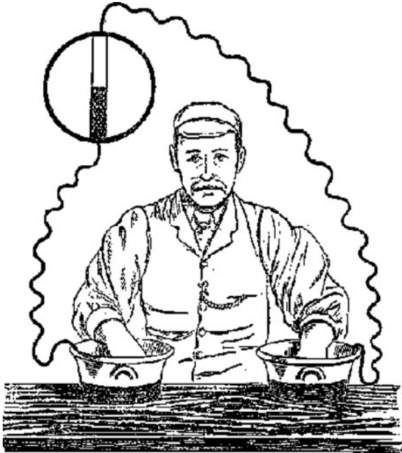
Fig. 3.14 Human subject connected to capillary electrometer via large area “bucket” electrodes [141]
