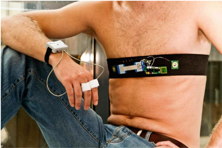
Fig. 8.8 Integrated body area network for ambulatory monitoring of physiological responses from the Autonomic Nervous System
