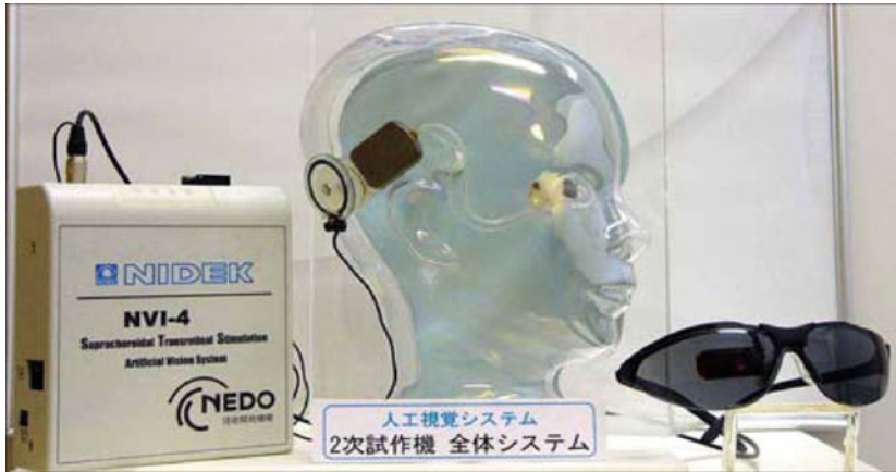
Fig. 14.8 A mock-up system of STS-based retinal prosthesis. Courtesy of Nidek Co. Inc
