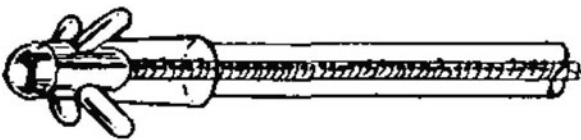
Fig. 3.46 Transvenous lead with silicone rubber tines [132]
