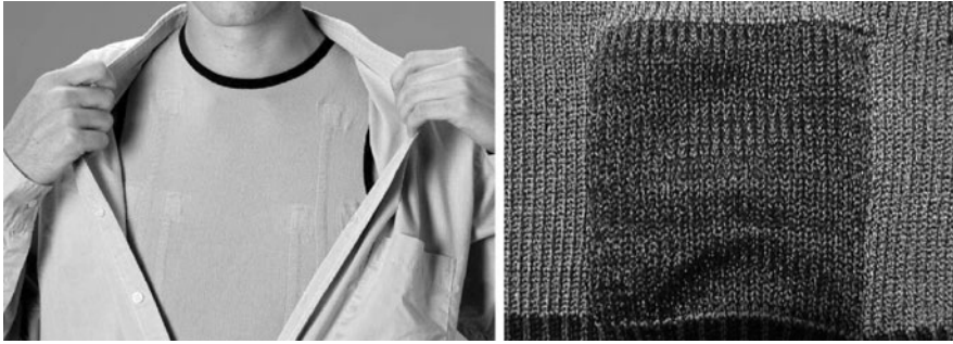
Fig. 3.27 a: The WEALTHY physiological monitoring vest with integrated sensors b: An early version of the “fabric” electrodes
