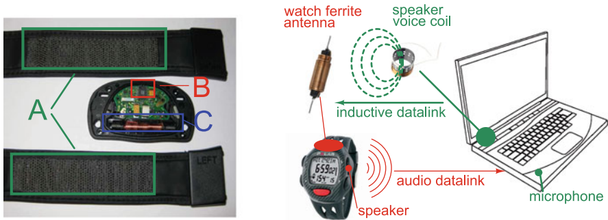
Fig. 7.39 On the left : Polar heart rate monitor chest belt with ECG electrodes (A), circuit board with ECG frontend and near-field transmitter (B) and ferrite antenna (C). The bidirectional data PC communication principle for Polar HRM is depicted on the right
