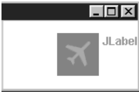
Figure 5.3 Demonstrating a disabled icon using GrayFilter
