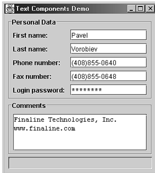
Figure 11.9 Example demonstrating the use of custom Formats with JFormattedTextField , and the use of InputVerifier to control focus transfer based on content validation
