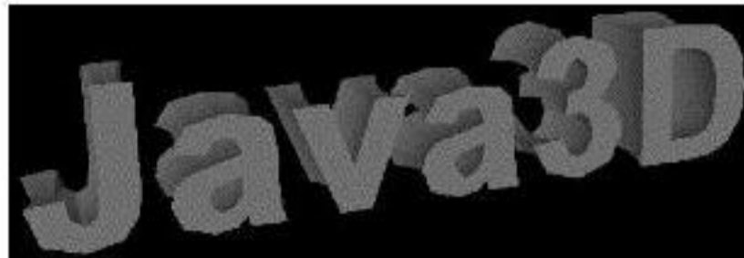
Figure 6.17: Same Text3D as in Figure 6.16 but with a tessellation tolerance of 1.0 specified in the Font3D .
