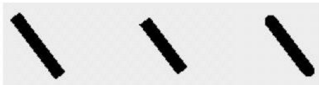
Figure 3.17: Cap styles in the BasicStroke class. From left to right: CAP_SQUARE , CAP_BUTT and CAP_ROUND .
