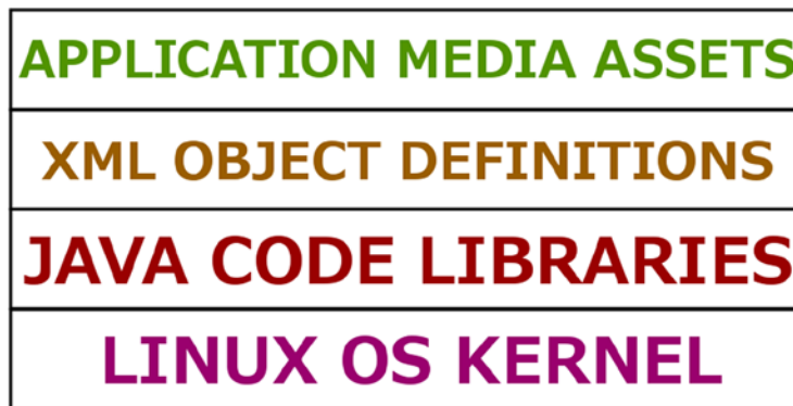
Figure 3-1. Android OS hierarchy, from Linux Kernel, to Java Libraries, to XML Definitions, to New Media Assets
