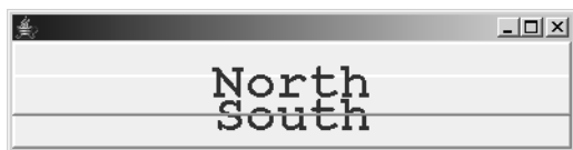
Figure 5-11. BorderLayout vertically resizes the NORTH and SOUTH components as the container height changes.
