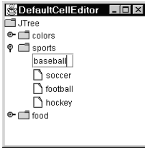
Figure 7-20. Double-clicking a tree cell with editing enabled causes a text field to appear in which the cell's text representation is displayed and can be edited.
