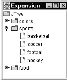
Figure 7-29. Selecting a node with children doesn't cause those child nodes to also be selected.
