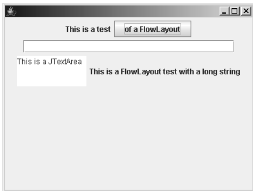
Figure 5-3. An example of how components appear when center aligned with FlowLayout
