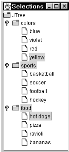
Figure 7-31. Expanding the selected node reveals that its children weren't selected as part of the range selection.
