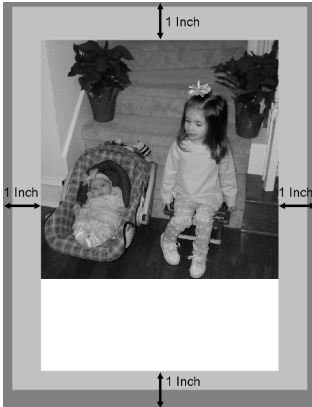
Figure 10-9. Scaling lets you take advantage of the imageable area without having a portion of your output clipped.
