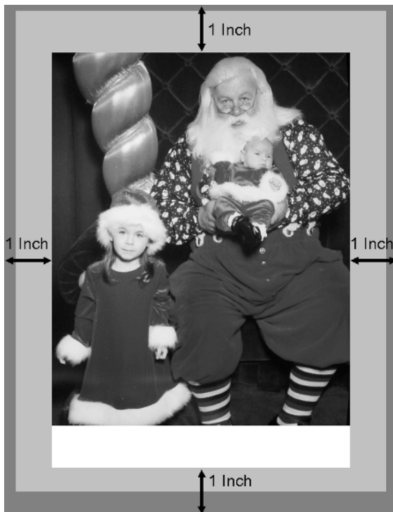
Figure 10-7. By using the translate() method, you can perform your drawing as if the upper-left corner of the imageable area corresponds to the coordinates 0, 0.
