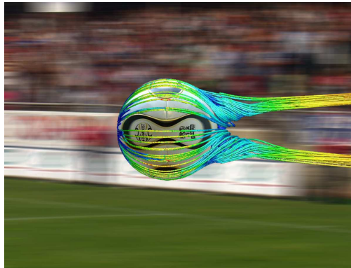
Figure 1.5: High speed airflow path lines colored by local velocity over the 2006 Teamgeist soccer ball.
