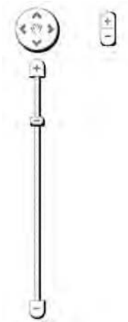
Figure 4-9. The default appearance of the navigation control. To the left is the big version and to the right the small one.
