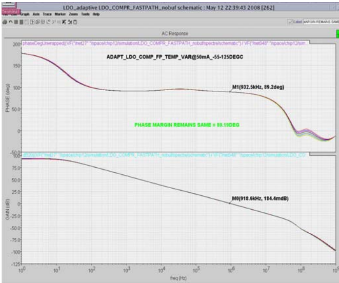
Fig. 9 Compensated LDO ac response at different temperatures (-55 to 125°)
