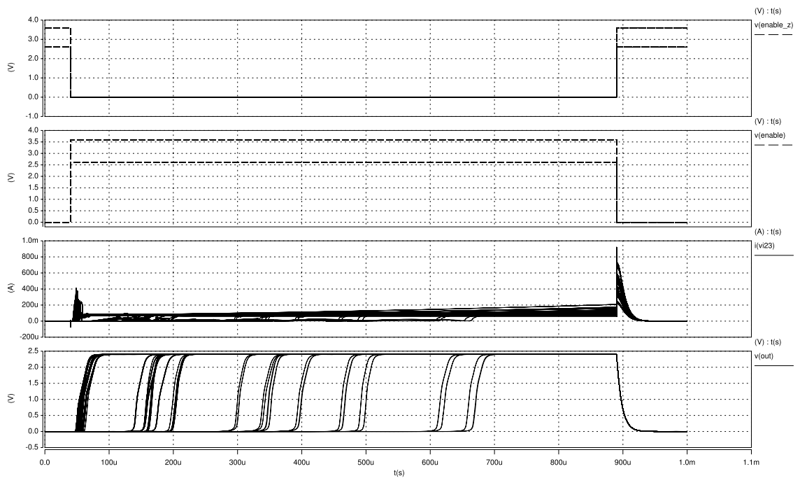
Figure 5.19: Power-Consumption performance of the power-down mode over all alters condition.
