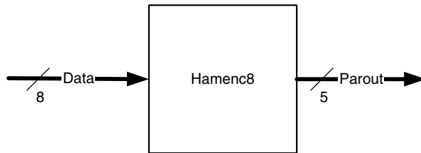
Figure 7.18 An 8-bit Hamming code encoder.
