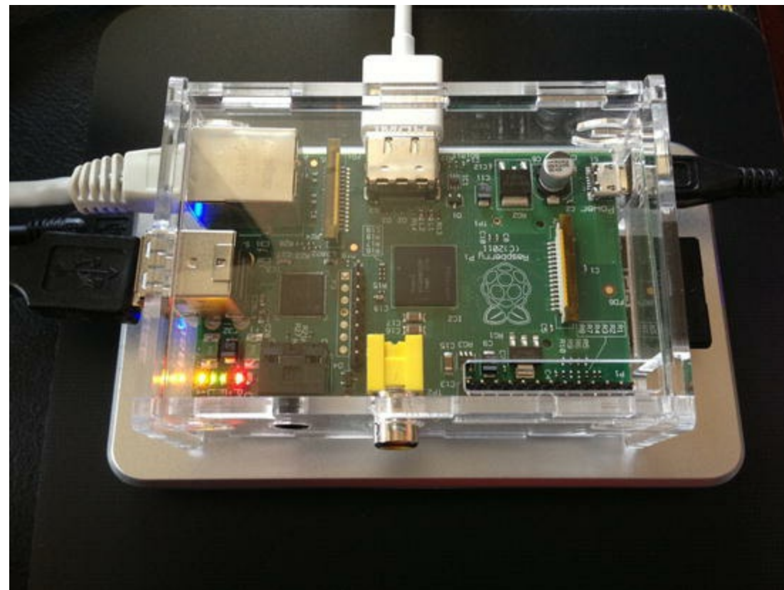
Figure 6-1. Raspberry Pi database server with an external drive 12
