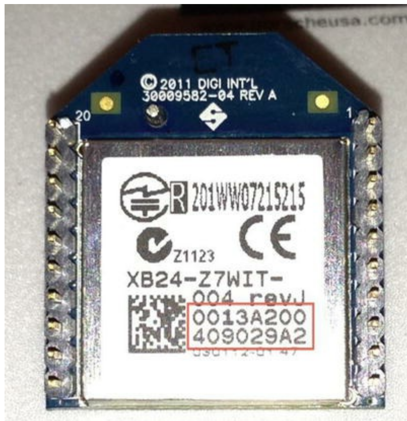
Figure 2-6. XBee address printed on the back of the module
