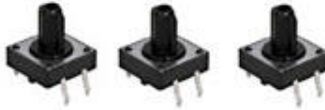
Figure 4.2. S.P.S.T. momentary, normally open. 0.48" square x 0.18" body. Plunger stands 0.3" above body. Four PC leads on 0.2" x 0.5" centers. CAT# MPB-127, http://www.allelectronics.com .
