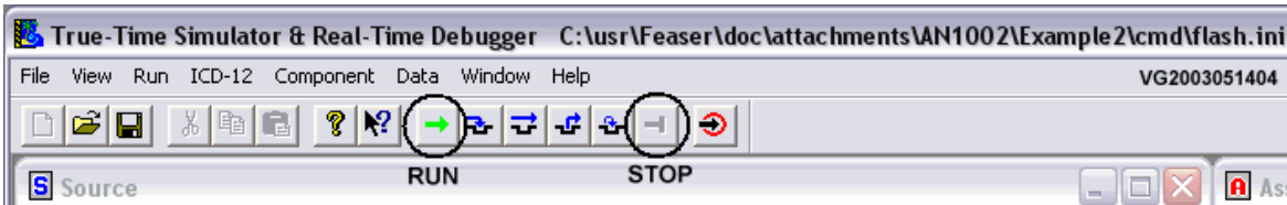
Figure 8 - Running and stopping your software application
