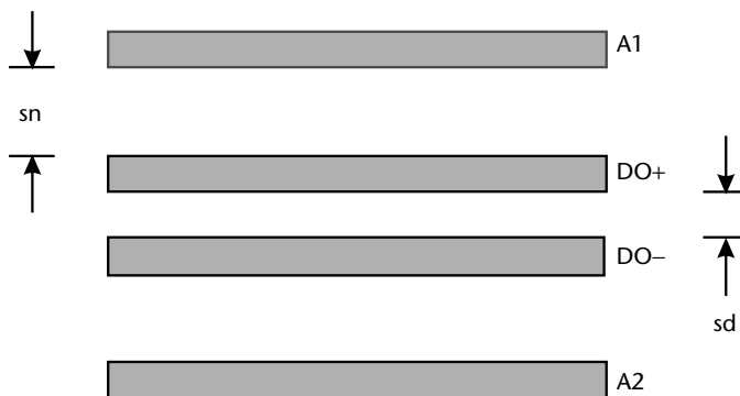
Figure 13.14 Top view showing four traces. Prevent common mode noise by making the spacing between the diff-pair ( sd ) smaller than the spacing to other traces ( sn ).
